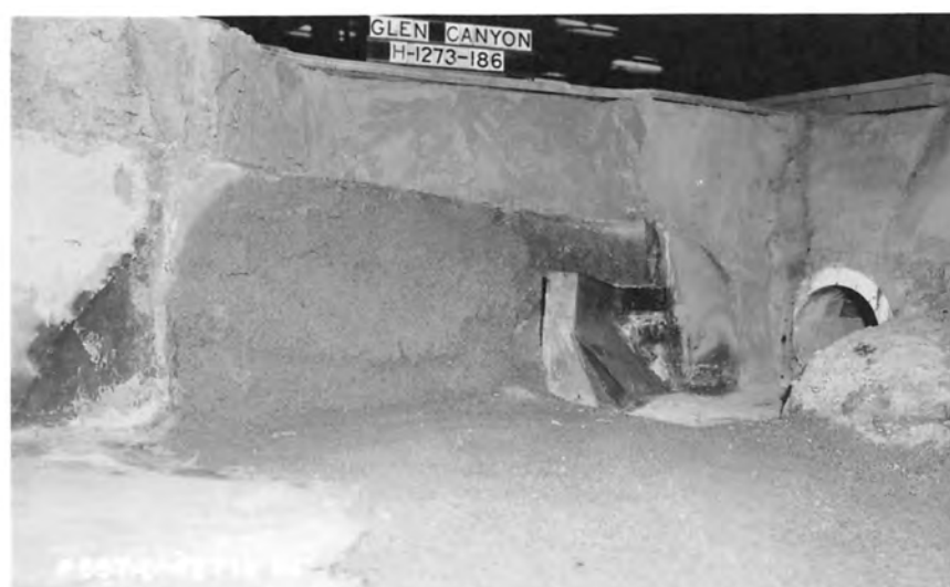
Superelevated extension wall downstream from deflector wall.
