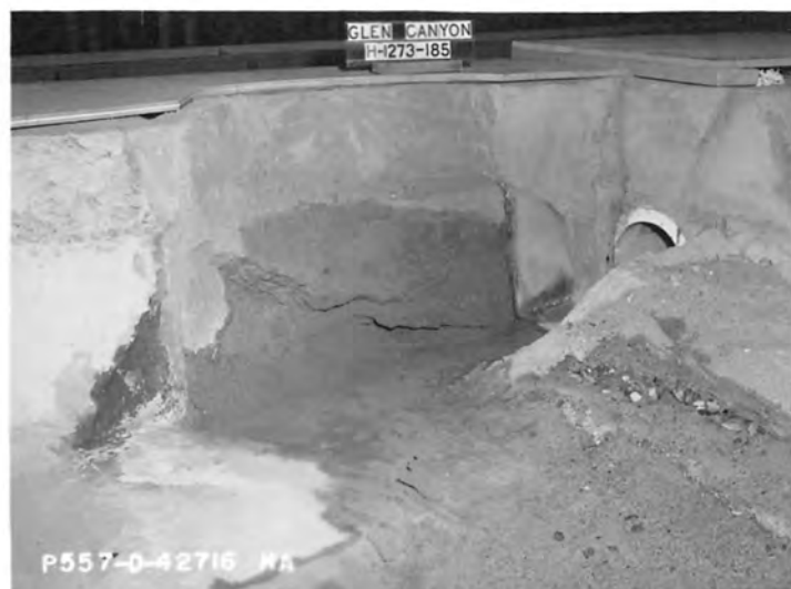
Extent of canyon wall erosion after 30 minutes operation at 50,000 cfs.
