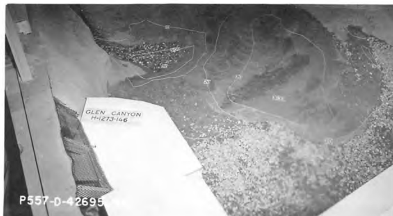
Erosion after 7 hours operation. Valves 3 and 4 discharging 7,500 cfs, 24,000 cfs thru powerplant. 32,000 cfs thru left spillway. About 5,000 yards of material moved into afterbay.
