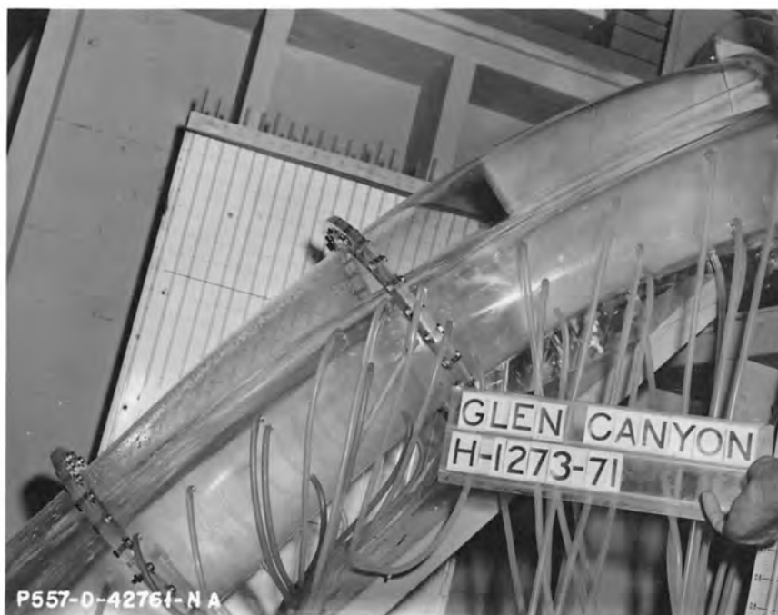
Flow in transition. Note small surface fin.
