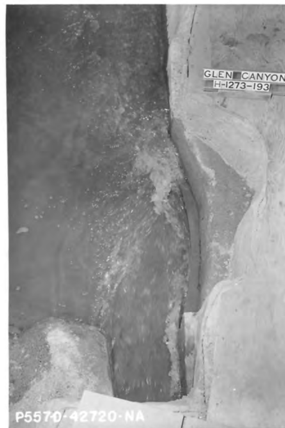
Jet deflected by tailwater surging.
