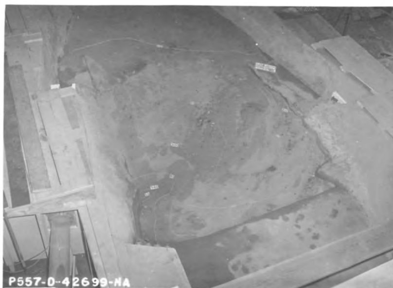
Erosion after 3 hours (model time) operation at 15,000 cfs.
