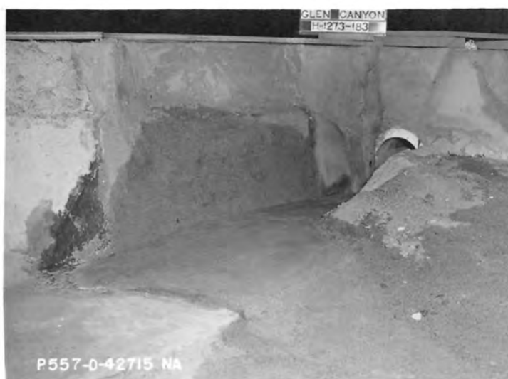
50-foot long deflector wall on right side at tunnel portal. Canyon wall and riverbed molded in erodible sand-cement mixture.
