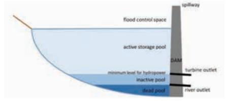
Figure V(D)(2)-3. Typical distribution of reservoir water allocation between active storage, inactive storage, and "dead pool," with a portion of the reservoir storage reserved for flood control purposes.
