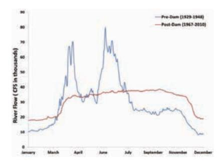
Figure III-13. Altered Stream Hydrograph. Hydrograph of the Missouri River hydrograph pre- and post-dam construction, showing effects of dam operations on the timing and volume of natural stream flows. Source: NRDC (2014).
