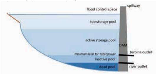
Figure V(D)(2)-8. Distribution of reservoir water allocation with "top storage" pool for carryover storage space.
