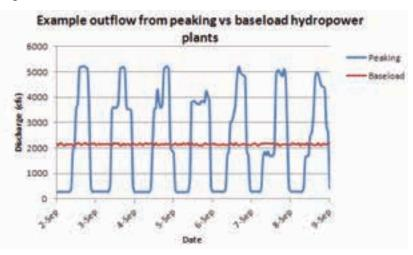
Figure III-14. Daily Hydrograph Downstream of Hydropower Dam. Hydrograph showing character of dam discharges when hydropower dam is engaged in peaking power production versus baseload production. Source: Oregon State University (2014).
